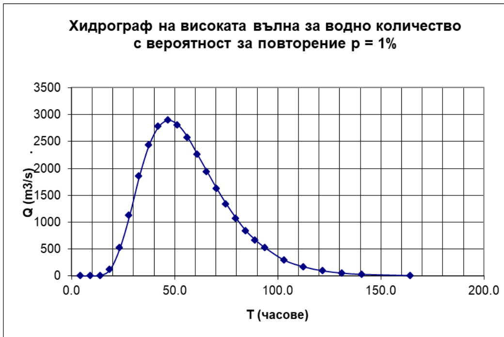
Figure 7: High wave hydrograph used in the computational model
